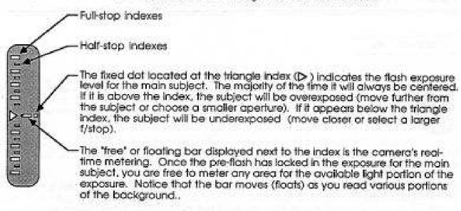
If the bar is above the triangle index, the background will be overexposed relative to the main subject. If it is below the index, the background will be underexposed. If it is lined up at the triangle index, both background and main subject will be correctly balanced.
